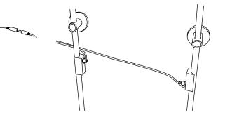
OPTIONAL: To connect multiple rail sets, mount the additional rail set a maximum of 15.7 in. away. Use rail extension cables to connect additional rail kit section; ensure the polarity is being respected (red left/blue right).
