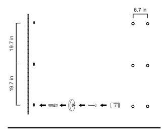
Insert rail into support. Tighten the allen set-screw, located on the support, when rail is in correct position. Repeat this step when connecting additional rails.
