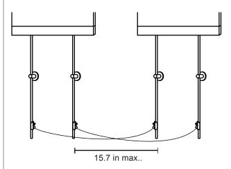
Note: Longer connector cord may be required for increased distance between wall rails.
